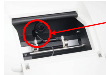
Sample chamber with built in temperature probe
